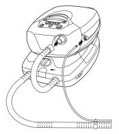
**5** Connect the mask system to the free end of the long air tubing. The final assembly should look like this:
